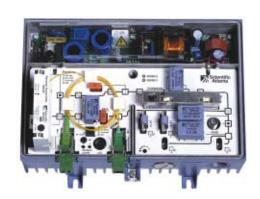
level, and a plug-in interstage equalizer for RF tilt. A directional coupler RF test point is provided at the forward output and reverse transmitter input, allowing for accurate signal level measurement. Surge protection is provided for the RF ports, and all Compact products are equipped with a double gasket that includes an RF and a water-dust gasket.
